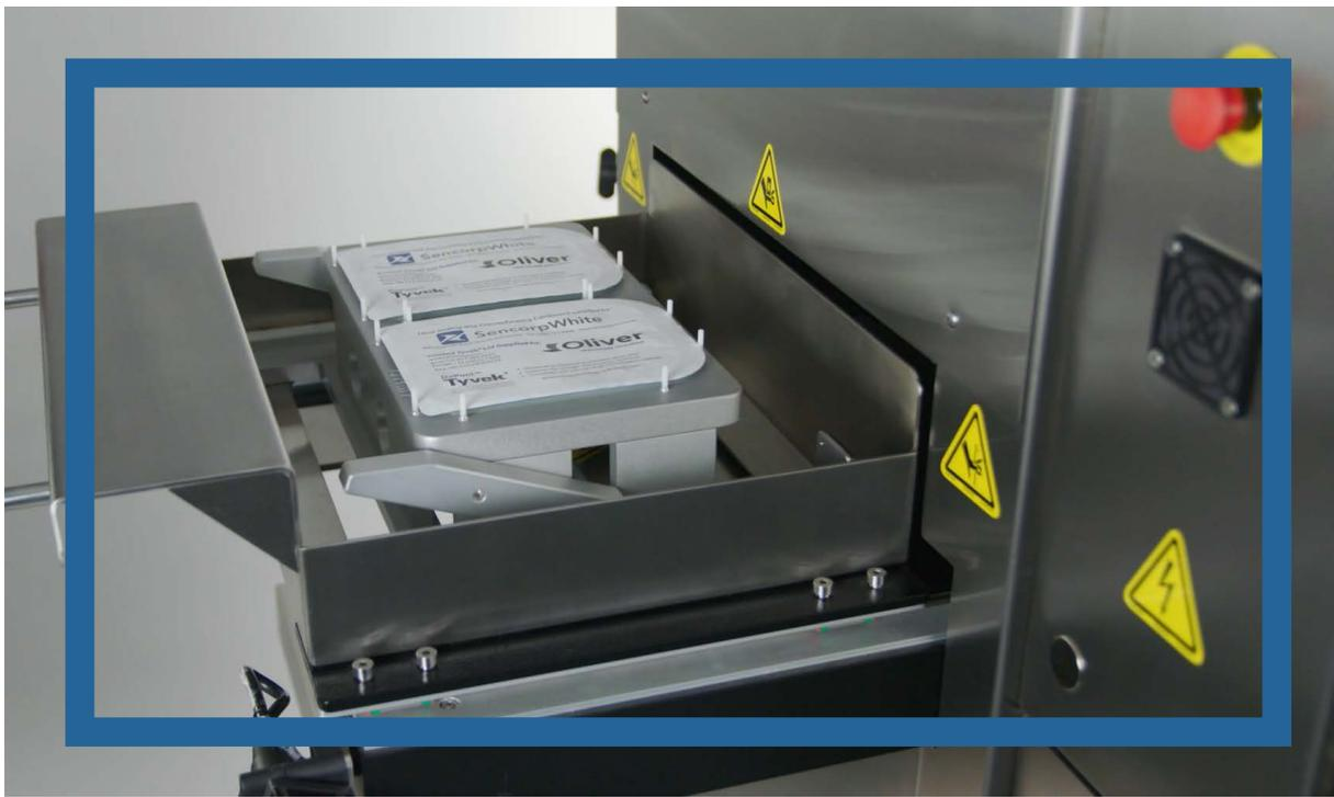
By contrast, tray sealing completely bonds the lid to the tray, enabling a hermetic seal. In addition, these products are typically higher-value medical devices, such as joint replacements and implants, that need to be packaged so that they are immobilized and yet readily accessible and presentable in medical settings.
